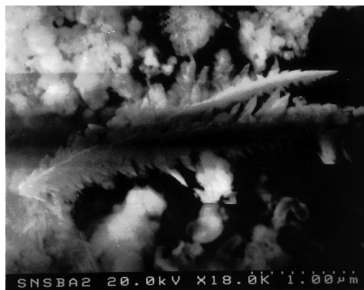
Fig. 2 SEM image of SnSb alloy prepared by reductive co-precipitation in ethanol solution at 0.0–1.0 °C with ultrasonic treatment (sample E). A feather-like particle with two branches can be seen in the center region.
